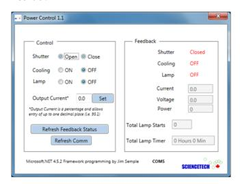
Software GUI for power supply control
