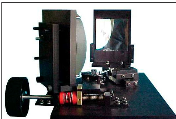
Variable Focus Mechanism on a 1kW Solar Simulator
