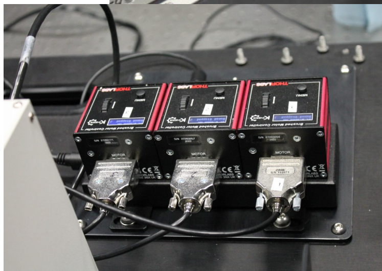
Motorized Slit actuator controllers mounted on TLS System
