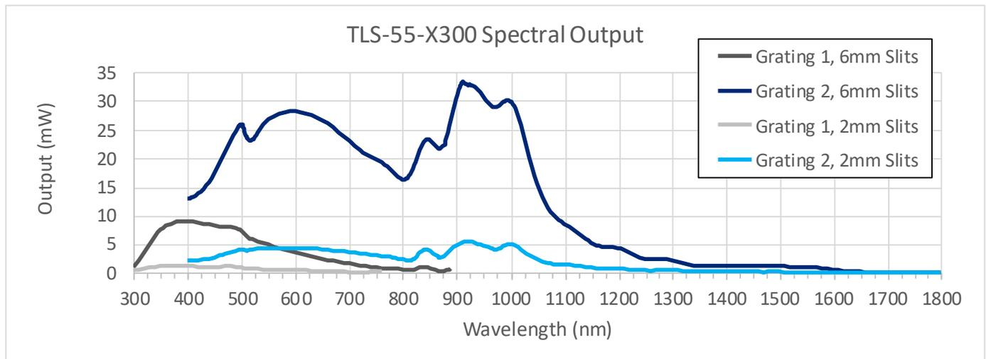
Typical output power of the TLS-X55-300 (Xe lamp 300 W) with various gratings and slits
