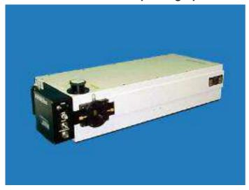
The Sciencetech 9057 is a half meter motorized Czerny-Turner monochromator (and spectrograph) with an f/8 aperture. A "faster" model with larger optics for higher light throughput is also available as the 9057Fwith f/5.9 aperture. Both models have a computer controlled motorized turret for automatic grating and wavelength selection. The regular 9057 model supports up to three 50 x 50mm gratings whereas the larger optics 9057F model supports up to two  $64 \times 64$ mm (clear aperture) gratings.
